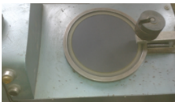
Fig. 3. Installation of testing abrasive wear with abrasive disc
